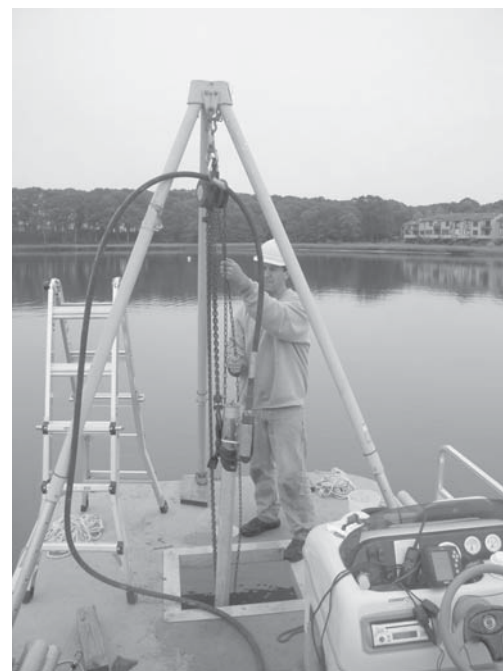
A specially designed pontoon boat is used to extract core samples. Photo courtesy MapCoast.
