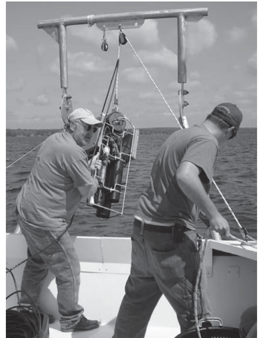
Above: BayMap researchers deploy the Sub-Chem Systems nutrient analyzer. This instrument measures nitrate, nitrite, ammonia, phosphate, iron, dissolved oxygen, salinity, and temperature at various depths in the water column. Photo courtesy BayMap field team.
