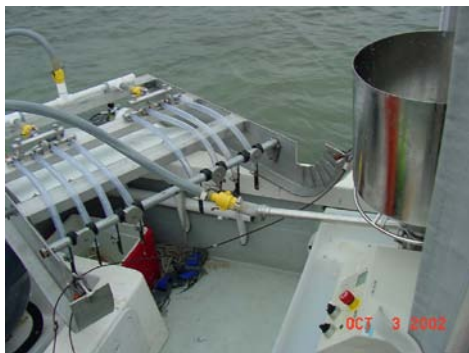
Eelgrass seeding sled is connected to the pump and seed/gel reservoir by a reinforced tube.
