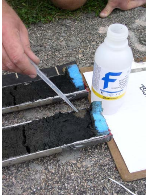
Figure 9: Applying hydrogen peroxide to a reduced soil
