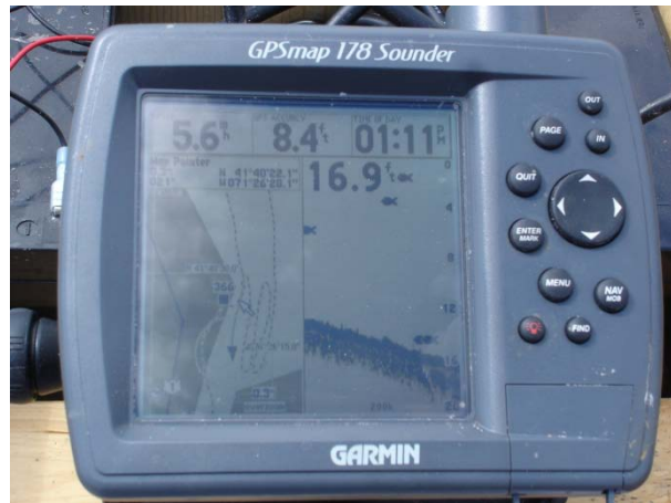
Figure 6: A Garmin echosounder collects and stores both depth (z) and location (x,y) data.
