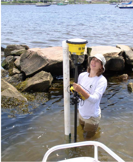
Figure 3: Measure elevation of tide gauge in order to tie depth measurements to a known elevation datum (NAVD88)
