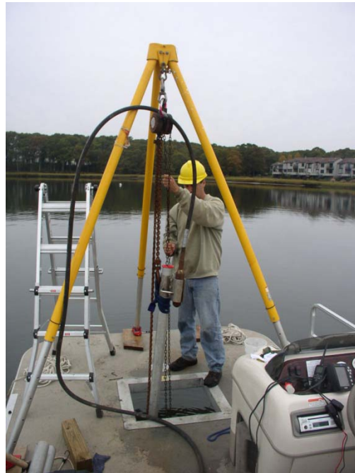
Figure 7: A vibracore set up using a tripod and chain-fall to extract a core through the “moon pool” of a pontoon boat.
