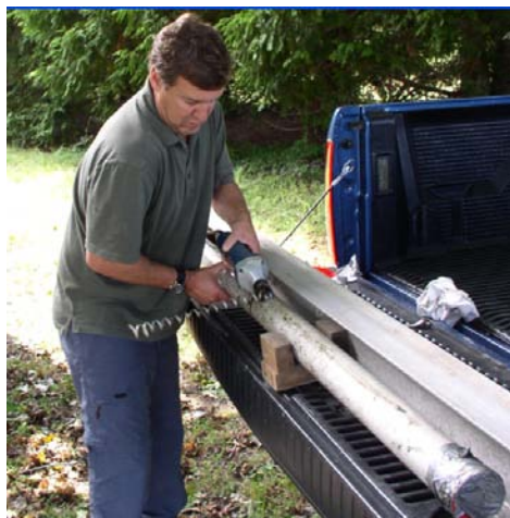
Figure 8: Cutting a core with electric sheet metal shears.
