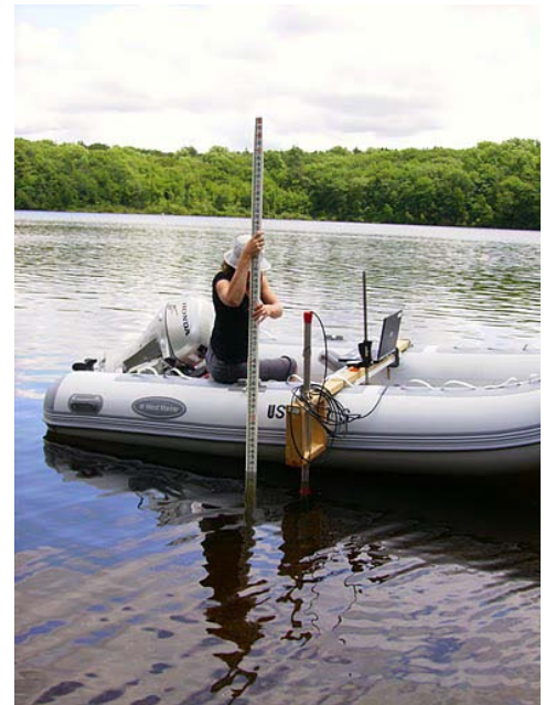
Figure 4: Manually check fathometer reading and determine offset
