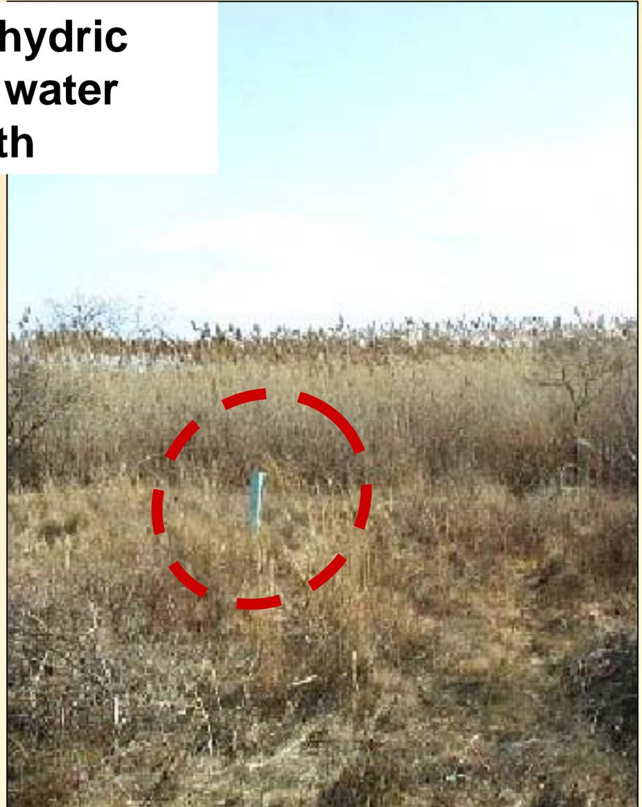
Ground water table test pipe for septic system suitability determination
