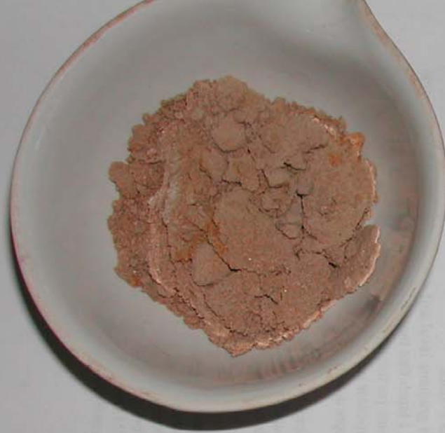
BhsM over bedrock. Note Fe concentrations.
