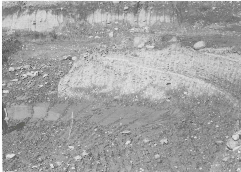
Fig. 5-5. Silt and clay beds (light colored bands) in the Lower Till at Barre (Site 3) (a). Rod in center of photo is 1.3 m long. Fig. 5-5 continued on p. 86.
