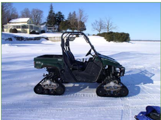
Yamaha Rhino tracked vehicle used for motorized GPR survey on frozen lake surface. The GPR antenna was dragged behind on a wooden sled. The ice was up to 24 inches thick.
