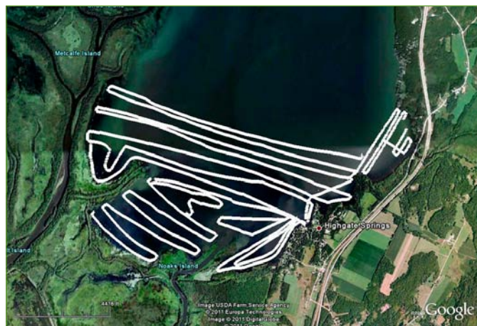
The location of GPR traverse lines completed over the southeast portion of Missisquoi Bay in northwestern Vermont.
