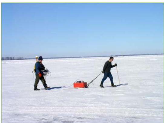
Roger DeKett pulls the 200 MHz GPR antenna while Jim Doolittle monitors data collection during an on-foot GPR traverse on Missisquoi Bay, Vermont.
