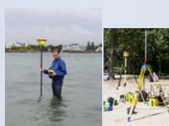
A survey grade (RTK) global positioning system is used to collect elevation data in shallow areas where traditional acoustic devices do not work. All elevations are tied to MSL based on NAVD 88.
