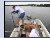
The bucket auger was used off the side of the boat for sampling subaqueous soils.
