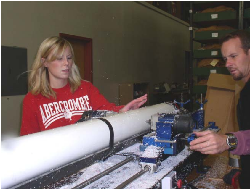
Left: a core cutting device using dual routers. Right: sheet metal shears.
