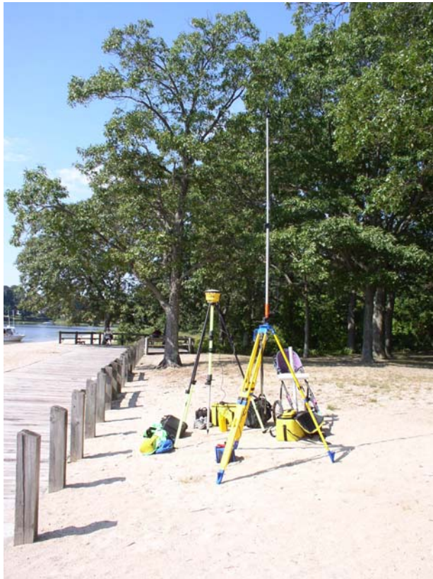
Left: 4800 setup, middle: rover interfaced with fathometer, right: Tide Gauge.
