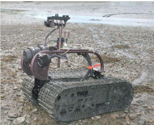
Wide track with external instrumentation mounts
