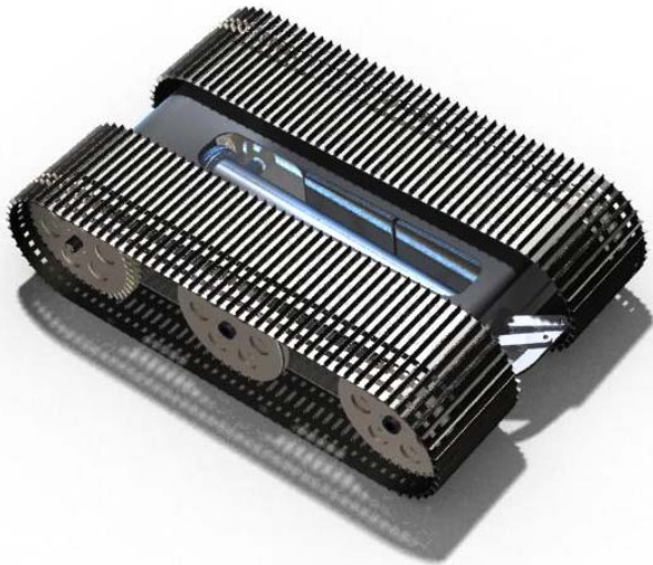
Wide track with interior alley for smooth profile, low ground pressure
