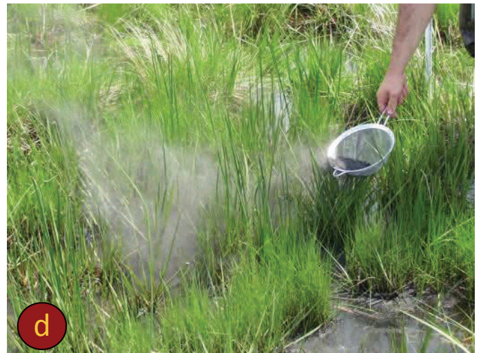
Fig. 4. Biomass was dried at 40°C for 24 hours and ignited in galvanized steel bins (a) (b) (c); After combustion, the ash was homogenized and spread evenly over the Ash Deposition plots using a 1-mm mesh sifter. This ash was deposited on the soil surface of the Ash Deposition and Canopy Removal + Ash Deposition plots in April 2009 (d).
