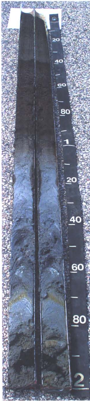
A soil core of a Billington silt loam soil. This core shows 4 major geologic events: glacial till (183–200 cm), loess (105–183 cm), freshwater organics (40–105 cm), and highly fluid marine silts (0–40 cm).
