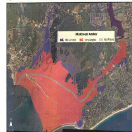
Fig. 3. A map of the mooring interpretation for mushroom anchors in Little Narragansett Bay based on the bottom type of soil material.
